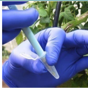
Eject sample into extraction tube
